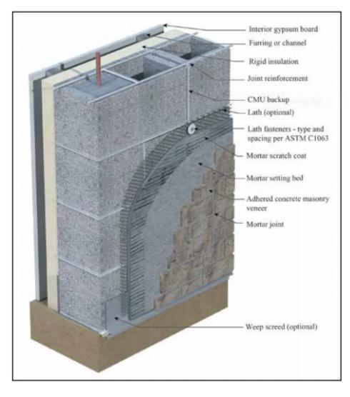
Figure 1-Application of Adhered Concrete Masonry Veneer Over Concrete
