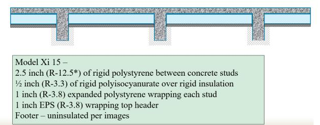
Figure 10: Superior Walls Model Xi 15 Insulation Summary
