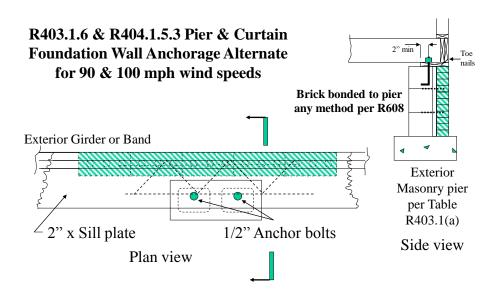
Max pier spacing limited to girder span or 12'-0", whichever is less
