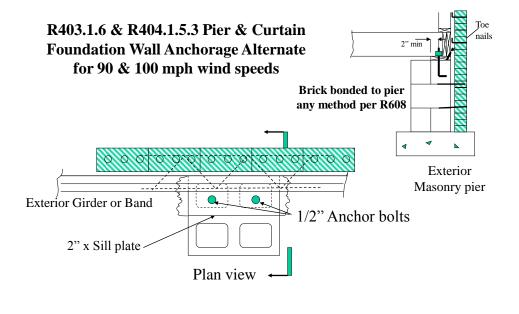
Keywords: Foundation anchorage, pier & curtain wall foundations
