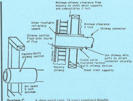
System C (6 inch Clearance) A sheet metal (min. 24 gage) ventilated thimble having two 1 inch air channels shall be used with a sheet steel chimney connector (min. 24 gage). Sheet steel supports (min. 24 gage) shall be cut to maintain a 6 inch clearance between the thimble and combustibles. The supports shall be fastened to the wall on all sides. Glass fiber insulation shall fill the 6 inch space between the thimble and the supports. The thimble shall be secured to the support.
