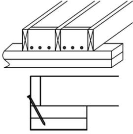
Blocking between rafters or truss not at the wall top plates, to rafter or truss
