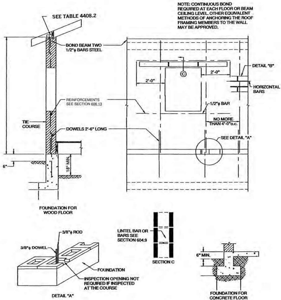
A FULL BED JOINT MUST BE PROVIDED. ALL CELLS CONTAINING VERTICAL BARS ARE TO BE FILLED TO TOP OF WALL. PROVIDE INSPECTION OPENING AS SHOWN ON DETAIL "A". HORIZONTAL BARS ARE TO BE LAID AS SHOWN ON DETAIL "B". LINTEL BARS ARE TO BE LAID AS SHOWN ON SECTION "C".
