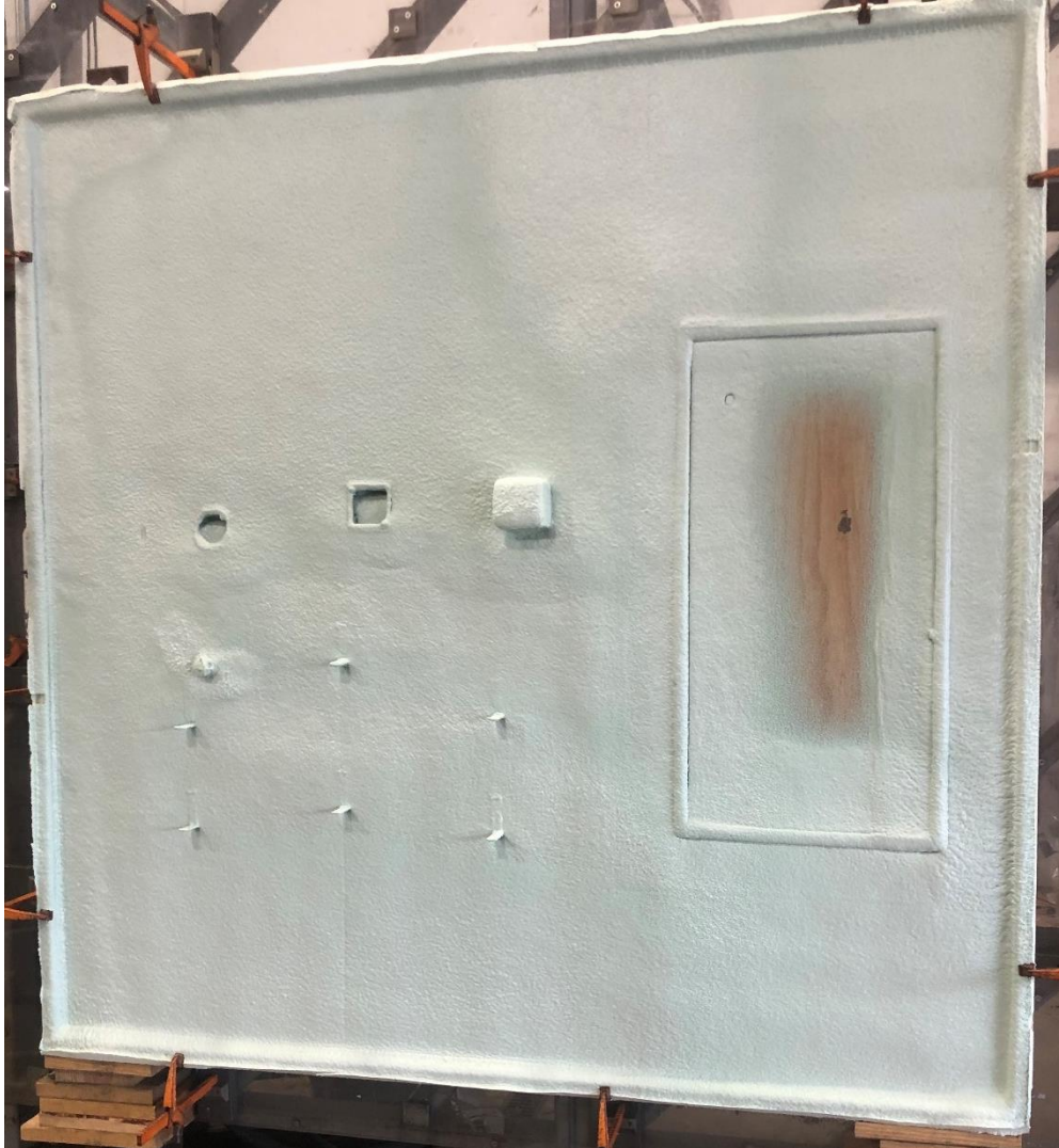
Photo No. 2 Penetrated Wall
