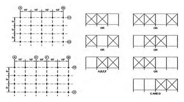
FIGURE R4603.6(e)(f)  ${\it ELEVATIONS} \\ ({\it SHOWING POSSIBLE ARRANGEMENT OF X-BRACING IN LINE}) (G~{\it AND H SIMILAR})$
