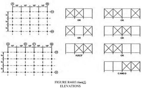
(SHOWING POSSIBLE ARRANGEMENT OF X-BRACING IN LINE) (G AND H SIMILAR)
