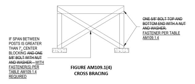
2018 NC Residential Code **ERRATA** – Figure AM109.1(4) corrected bracing location and lapping (200708).
