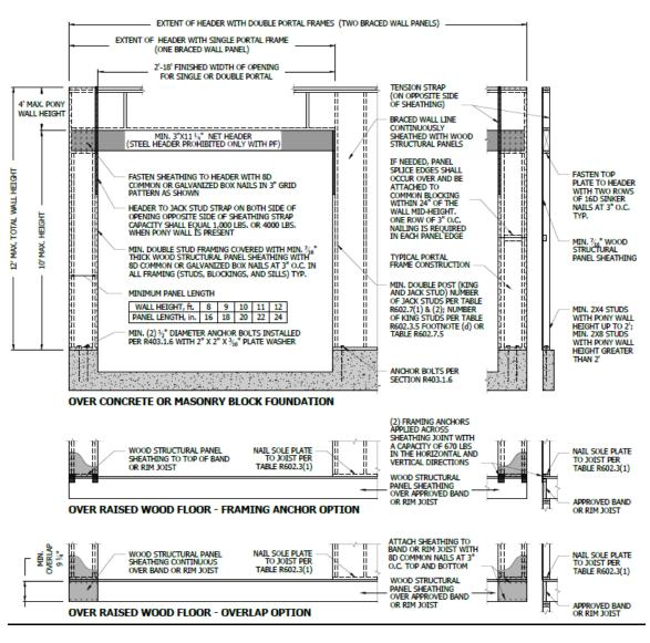
FIGURE R602.10.1 METHOD PF – PORTAL FRAME CONSTRUCTION
