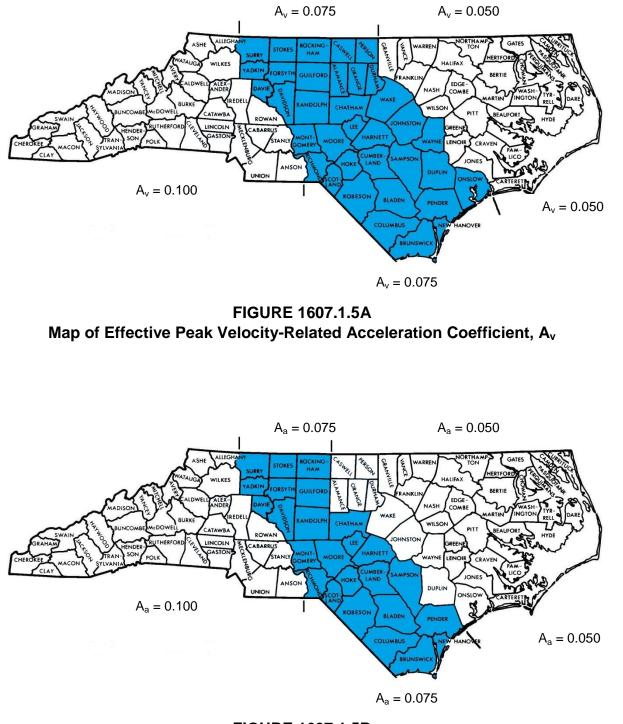
FIGURE 1607.1.5B Map of Effective Peak Acceleration Coefficient, A<sub>a</sub>
