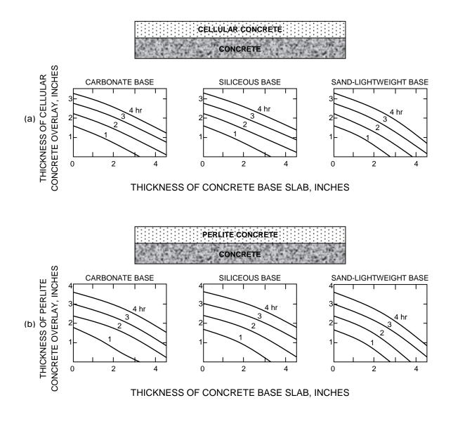
Figure 709.2.2B Fire Resistance Ratings for Concrete Floor Assemblies
