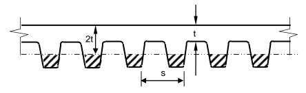
NEGLECT SHADED AREA IN CALCULATION OF EQUIVALENT THICKNESS
