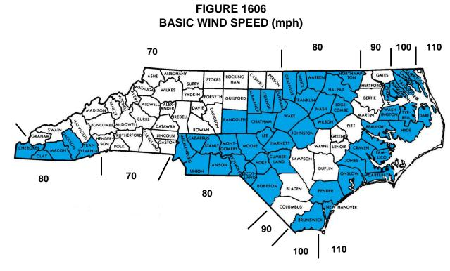
**Note:** The basic design wind velocity for the Outer Banks and parts of Carteret, Onslow, Pender, New Hanover, and Brunswick Counties on the seaward side of the Intracoastal Waterway shall be 110 mph.
