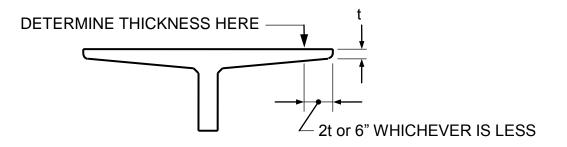
**709.2.1.1.5** The equivalent thickness of panels with ribbed or undulating surfaces shall be determined by one of the following expressions:
