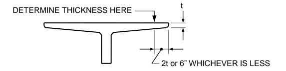
**709.2.2.1.4** The thickness of slabs with ribbed or undulating soffits shall be determined by one of the following expressions, whichever is applicable.
