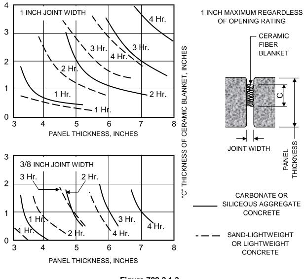
Figure 709.2.1.3 Ceramic Fiber Joint Protection
