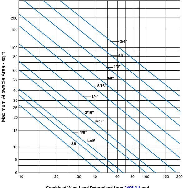
Combined Wind Load Determined from 2405.3.1 and Tables 2405.3A or 2405.3B in psf 1 sq ft =  $0.0929 \text{ m}^2$ 1 in = 24.4 mm 1 psf = 47.8803 Pa
