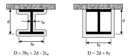
Figure 709.5.2 Determination of the Heated Perimeters of Structural Steel Beams and Girders
